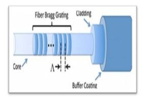
Fig 2. An Expanded View of an FBG
