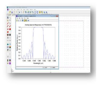
Fig. 14. Grating spectral response, i.e., relative power vs. wavelengthfor second simulation
