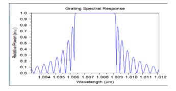
Fig 6. Simulation results from 1st grating analysis
