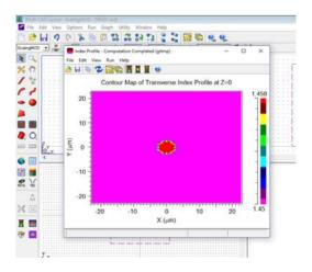
Fig 5. The computed index profile for a uniform FBG
