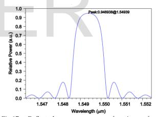
Fig.17. Reflected power as a function of wavelength with fiber having pitch 0.5323  $\mu m.$  Reflected power at 1550 nm is approximately 81.5 %
