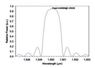
Fig. 19. Reflected power as a function of wavelength with fiber having pitch 0.5326  $\mu m.$  Reflected power at 1550 nm is approximately 91.5%
