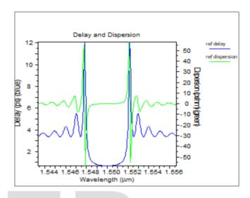
Fig 7. Simulation results from 1st grating analysis.
