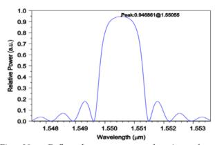
Fig. 20. Reflected power as a function of wavelength with fiber having pitch 0.5327  $\mu m$  . Reflected power at a reflectivity of 1550 nm is approx 81 %
