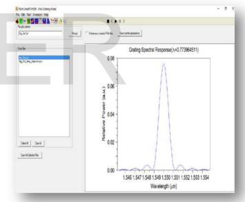
Fig.13. Grating spectral response, i.e., relative power vs. wavelength
