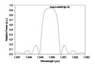
Fig.16. Reflected power as a function of wavelength at 1550 nm
