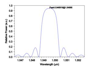
Fig. 18. Reflected power as a function of wavelength with fiber having pitch 0.5324 µm.
